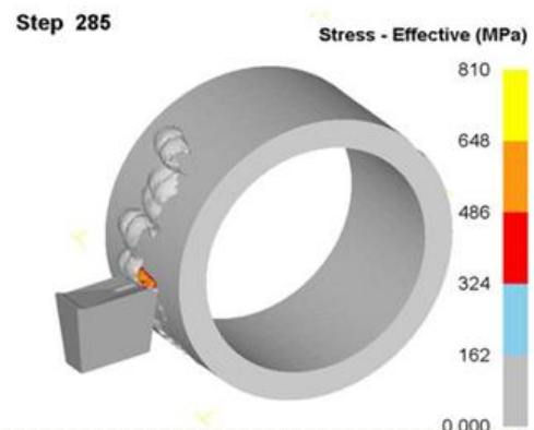
Figure 9. Effective stress of elliptical chip breaker.
